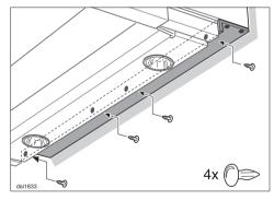
Secure the spacer strip to the back of the appliance from behind using 4 plastic rivets as shown.
